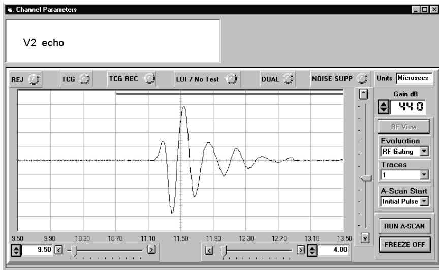
Figure 6. The A-scans from transducers H3 (a) and V2 (b) using the experimental setup shown in figures 2 and 3.
