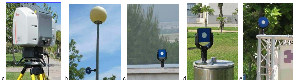
Figure 2: : a) Leica HDS ScanStation2 time-of-flight; b-e) artificial targets used for the survey
