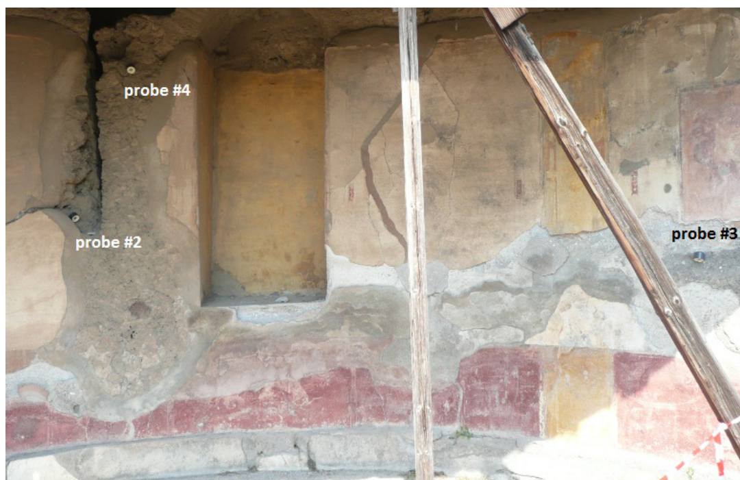
Figure 4.6: Location of probes #2, #3 and #4 in room 4. The picture was taken at 1:05 PM. The brighter zone at the lower right corner corresponds to sunlight incident on the frescoes that affects #3 from 2:00 PM to 8:00 PM.
