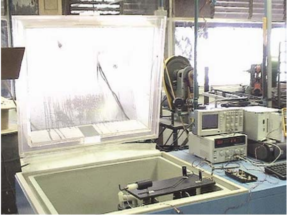
Figure 16. Photograph of the visibilimeter during calibration procedure.
