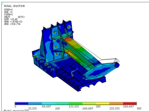
Fig. 12. FEM analysis for a bending test.
