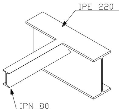
Fig. 2. Joint between IPE-220 strongback and IPN-80 cross girder.
