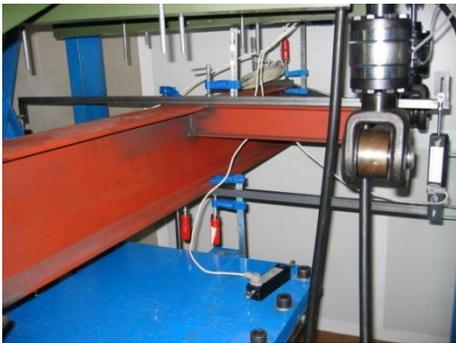
Fig. 7. Displacement sensors fixed to the test specimen.
