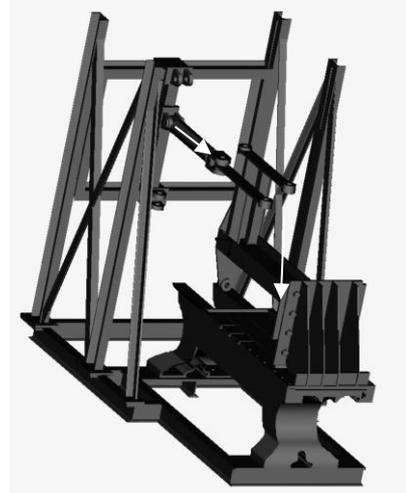
Fig. 11. Lateral bending on the cross girder.
