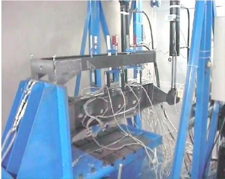
Fig. 6. Displacement sensors fixed to the anchor plate.
