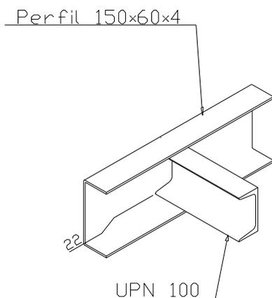
Fig. 3. Joint between U 150x60x4 and UPN100 cross girder.
