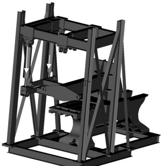
Fig. 8. Combined bending and torsion on the strongback.
