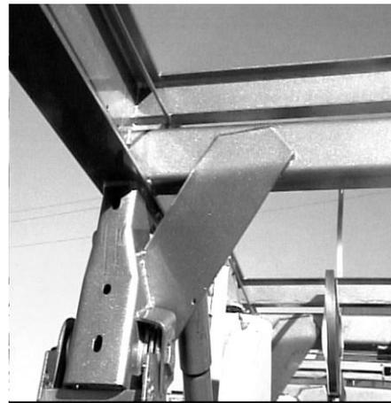
Fig. 4. Joint detail between frame and suspension.
