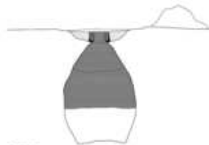
05 EXCAVATION OF STORAGE SPACE AND COVERING OF INNER SURFACES WITH LIME MORTAR
