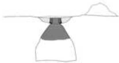
04 EXCAVATION OF STORAGE SPACE AND COVERING OF INNER SURFACES WITH LIME MORTAR
