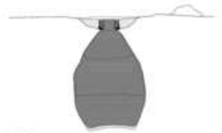
06 EXCAVATION OF STORAGE SPACE AND COVERING OF INNER SURFACES WITH LIME MORTAR (PHASE 3) SILO'S BASE COMPACTING
