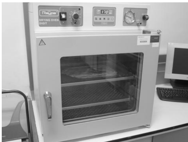
Fig. 14. Thermal treatment of a mat of PVA nanofibres at 170 \text{ }^\circ\text{C} in vacuum (250 mbar).
