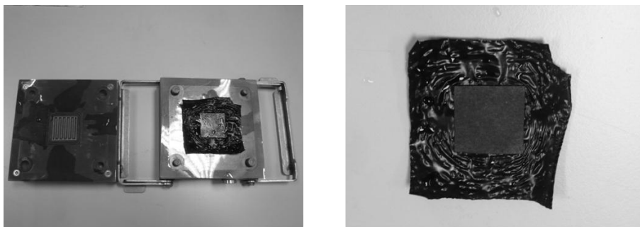
Fig. 23. Pictures of a prepared MEA containing a nanocomposite SPEEK-PVA/SPEEK-PVB membrane crosslinked at 120 \text{ }^{\circ}\text{C} . On the left, the 5 \text{ cm}^2 cell hardware used for DMFC experiments is also shown.
