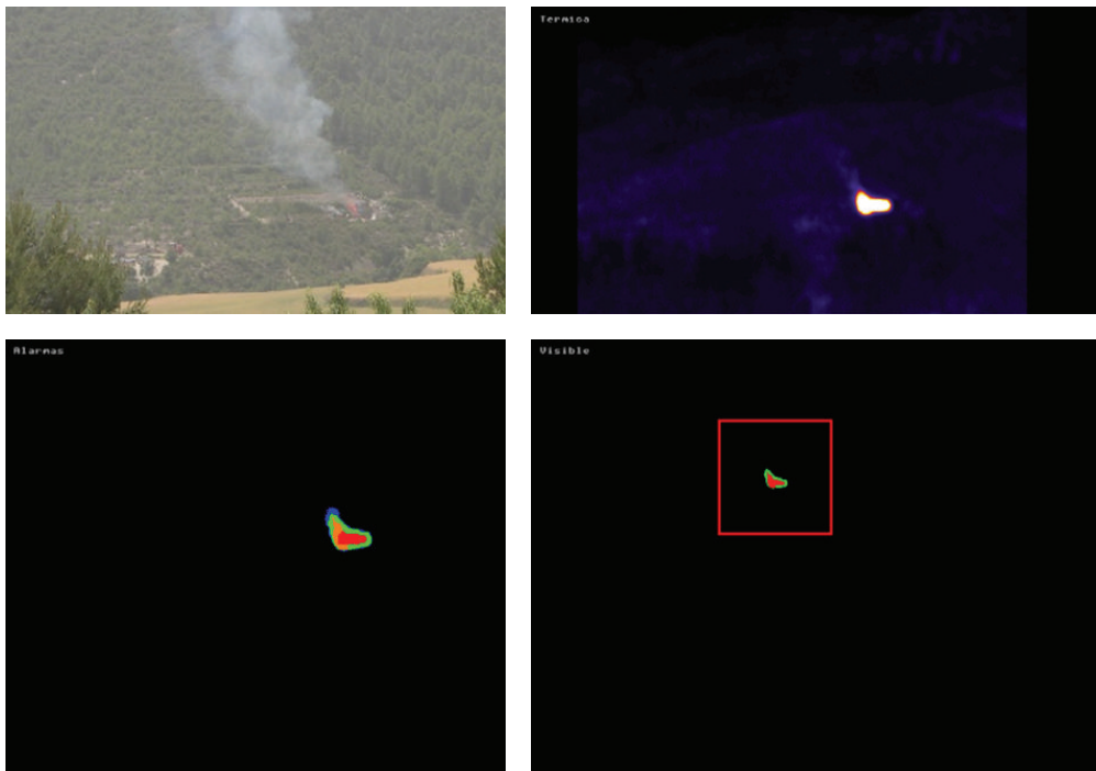
FIGURE 7: Example of controlled fire detection in real environment.
