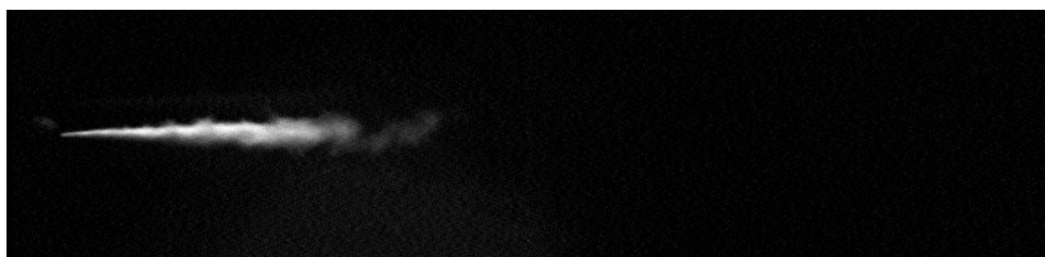
Figure 3.3. Sample image of the Mie-scattering technique at 1000 \mu s after SoI.
