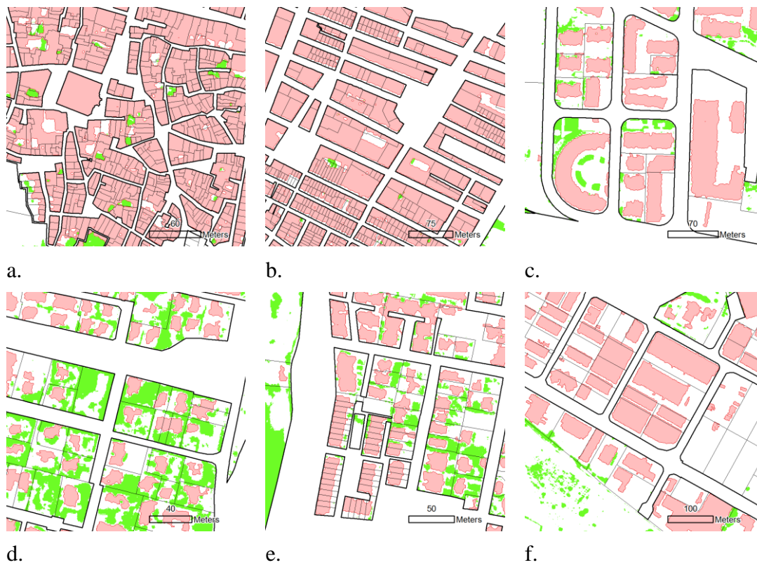
Figure 4. Examples of detected building (in pink) and vegetation (in green) for the defined urban classes: a. historical ; b. urban ; c. open urban , d. Detached housing ; e. semi-detached/terraced housing ; f. industrial .
