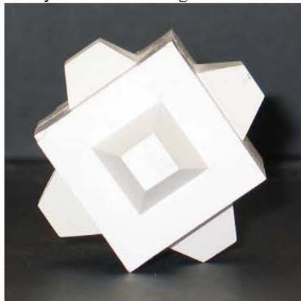
Figure 2. 3D view of Cubipod concrete armour unit
