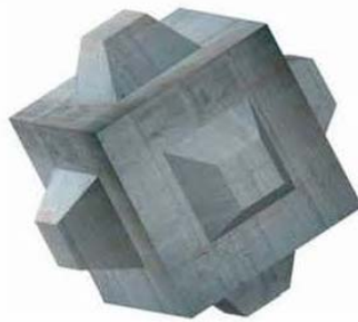
Figure 3. 3D view of the Cubipod.
