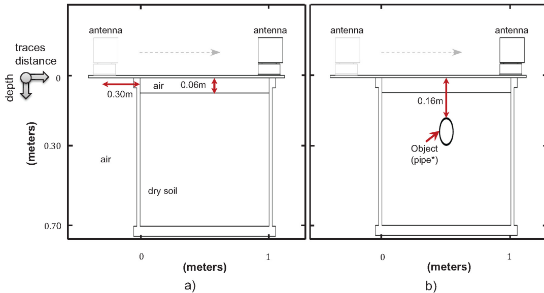
Figure 3.13: Schematic configuration for Case 1, experimental studies – Matrices T_{14} and T_{15} . (a) Capture for no-pipe – reference configuration –, and (b) capture for pipes' configurations
