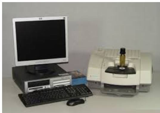
Figure 3.5. Picture of Nicolet Avator 360 FTIR spectrometer
