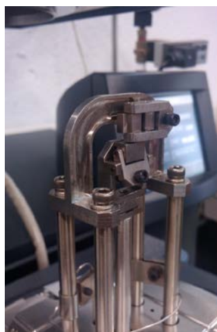
Figure 3.16. Picture of the TA Instruments DMA Q800 (left) and the tension mode clamp used in the measurements (right).
