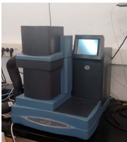
Figure 3.16. Picture of the TA Instruments DMA Q800 (left) and the tension mode clamp used in the measurements (right).
