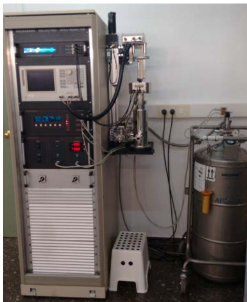
Figure 3.11. Picture of the Novocontrol Concept 80 instrument and the liquid nitrogen Dewar
