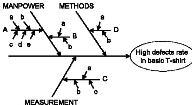
Figure 4. Cause and Effect diagram
