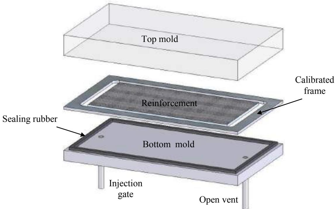
Figure 2 – Typical test mold as described in [23].
