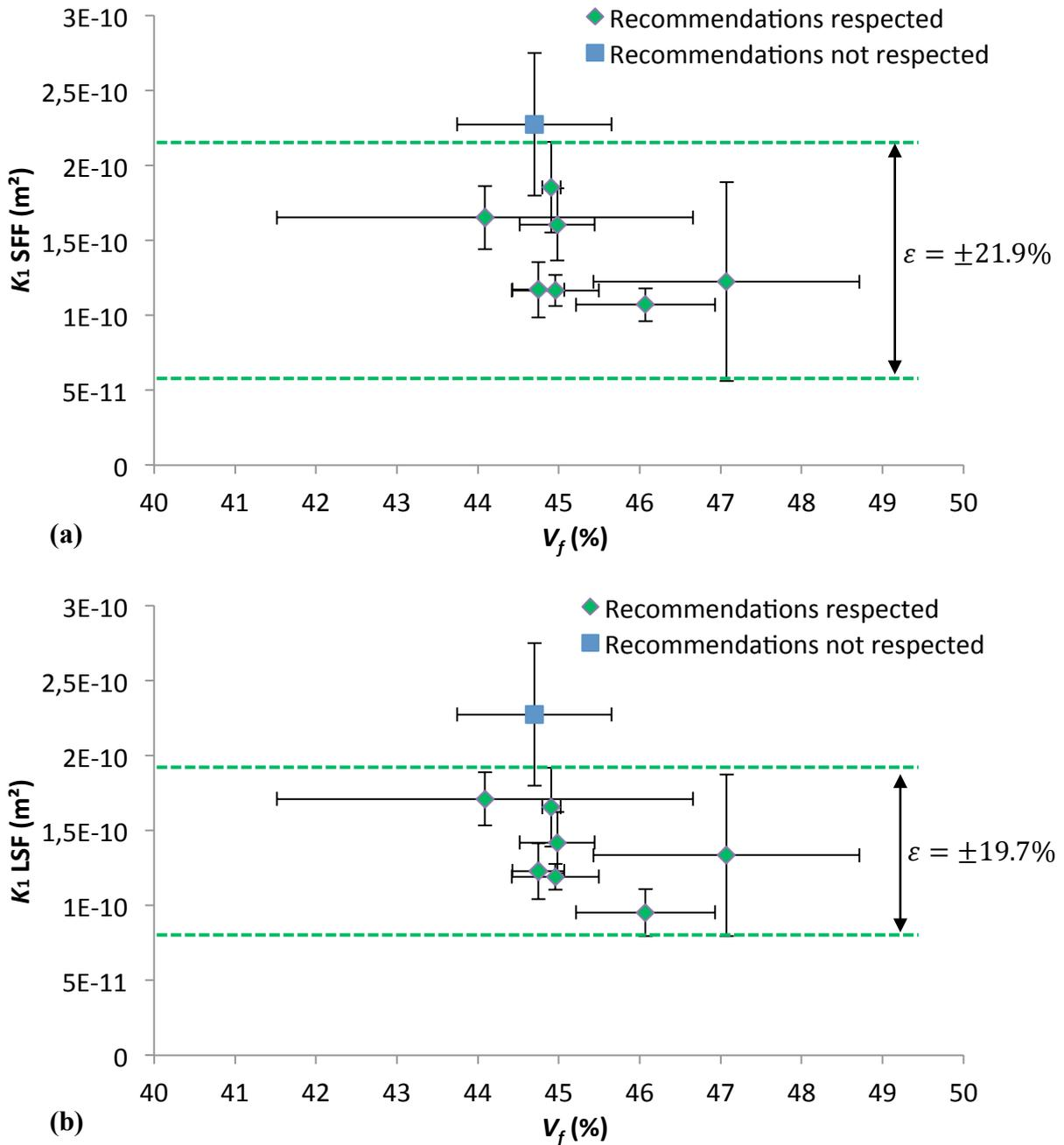
Figure 7 – Principal permeability  $K_1$  obtained using: (a) the SFF method and (b) the LSF method.
