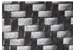
As displayed in Figure 1, testing directions at 0° and 90° were defined respectively in the warp and weft of the roll. The 45° testing orientation was obtained between the 0° and 90° counter clockwise. This upfront definition allows the comparison of the unidirectional effective permeability of all participants.
