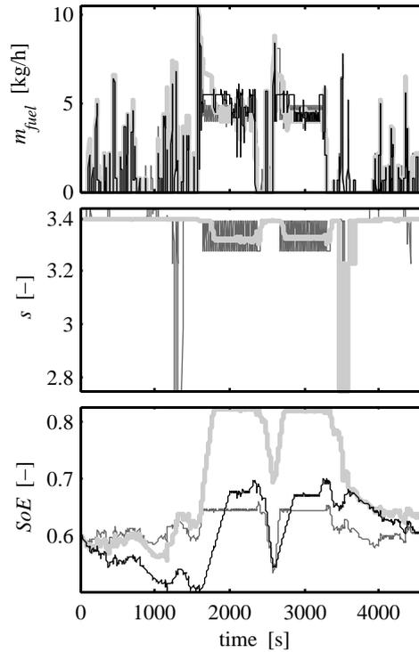
Figure 8: Evolution of the fuel consumption (upper plot),  $s$  parameter (middle plot) and  $SoE$  (bottom plot) with  $\beta=100$  s (dark grey) and  $\beta=500$  s (light grey). The black line represents the optimal solution obtained with DP.
