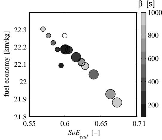
Figure 10: Fuel economy (km/kg of fuel) versus final  $SoE$  for different time horizons ( $\beta$ ) from black ( $\beta=100$  s) to light grey ( $\beta=500$  s). The marker size represents the receding horizon ( $\tau$ ) used to calculate the power probability distribution: 100 s for small markers, 200 s for medium markers and 300 s for big markers. White dot represents the optimal results obtained with DP.
