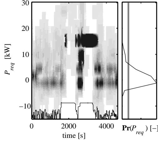
Figure 9: Evolution of the probability matrix during the tested cycle and qualitative representation of the vehicle speed. The colorscale represents the probability of a given required power at a given instant according to the probability matrix adaption, ranging from low probability in white to high probability in dark grey. Right plots show the probability distributions at the beginning (grey line) and the end of the trip (black line).
