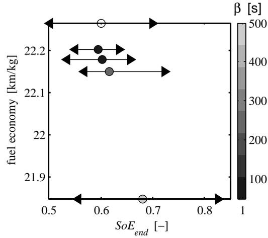
Figure 7: Fuel economy (km/kg of fuel) versus final  $SoE$  for different time horizons ( $\beta$ ) from black ( $\beta=50$  s) to light grey ( $\beta=500$  s). White dot shows the optimal results obtained with DP and arrows represent the range of variation of the  $SoE$  during the test.
