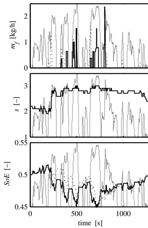
Figure A.12: Evolution of the fuel consumption (upper plot),  $s$  parameter (middle plot) and  $SoE$  (bottom plot) for a parallel HEV during an arbitrary driving cycle with the proposed adaptive method and  $\beta=100$  s (black line). The dotted line represents the optimal state of energy and fuel consumption evolution according to the DP solution.
