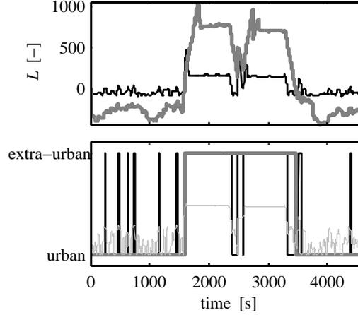
Figure 6: Evolution of the  $L$  parameter (upper plot) and detection of urban or extra-urban driving conditions (lower plot) with a sampling window ( $\kappa$ ) of 50 seconds (black line) and 250 seconds (grey line). The light grey line represents qualitatively the vehicle speed
