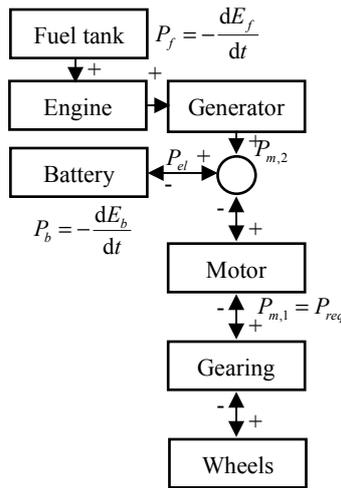
Figure 1: System layout, nomenclature and sign criteria for series hybrid architecture
