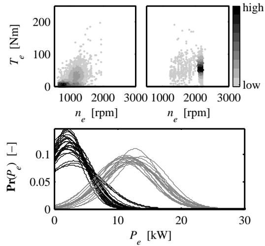
Figure 2: Upper plots: Operating points in the engine speed -torque ( $n_e - T_e$ ) map for urban (left) and extra-urban driving tests (right) and qualitative representation of its frequency  $\Pr(P_e)$ . Lower plot: Fit of the engine power ( $P_e$ ) during urban (black line) and extra-urban (grey line) tests to normal distributions
