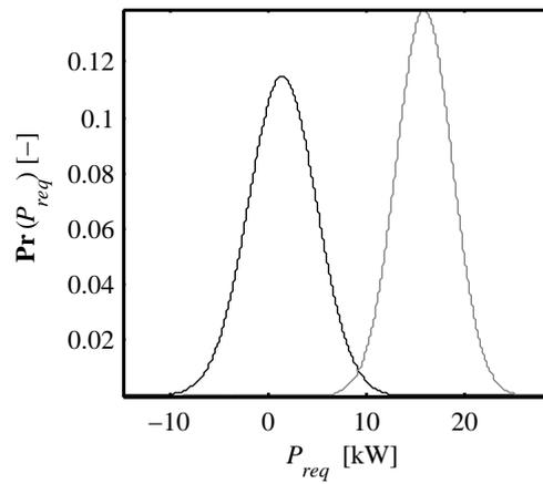
Figure 3: Fits of the power required by the vehicle ( $P_{req}$ ) during urban (black line) and extra-urban (grey line) tests to normal distributions
