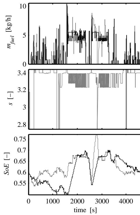
Figure 11: Evolution of the fuel consumption (upper plot),  $s$  parameter (middle plot) and  $SoE$  (bottom plot) with the adaptive method with  $\beta=100$  s and  $\tau=300$  s (grey line). Black line represents the optimal state of energy and fuel consumption evolution according to the DP solution.
