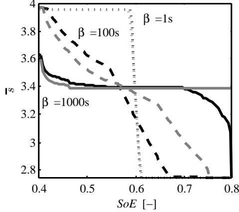
Figure 5:  $\bar{s}$  as a function of  $SoE$  to balance the battery energy consumption after  $\beta = 1$  s (dotted line),  $\beta = 100$  s (dashed line) and  $\beta = 1000$  s (continuous line) during urban (black line) or extra-urban (grey line) conditions supposing an initial  $SoE$  of 0.6
