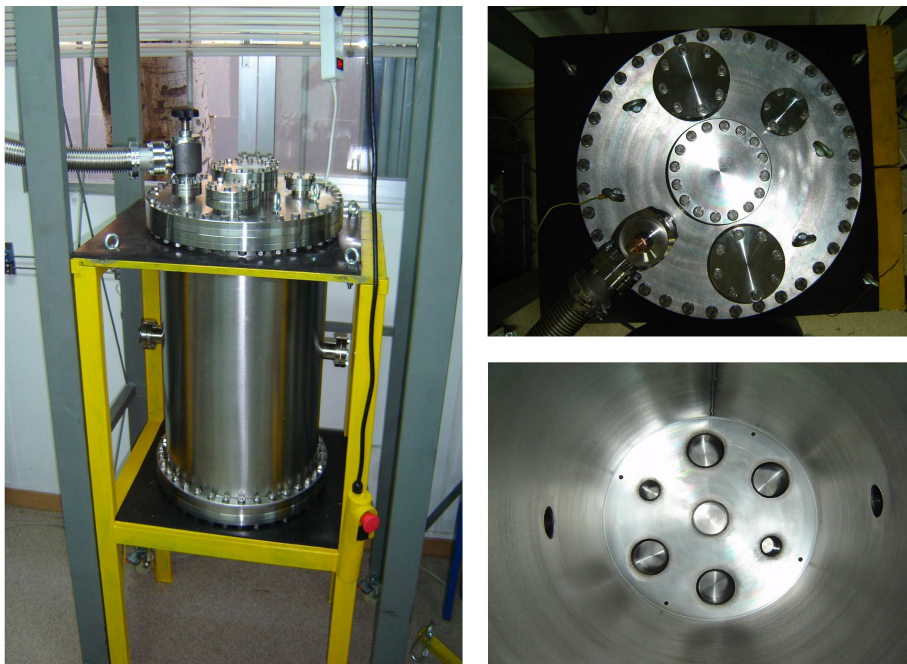
Figure 2. General view of the pressure vessel (left), external view of the upper cap (right top) and internal view of the vessel body and lower cap (right bottom).
