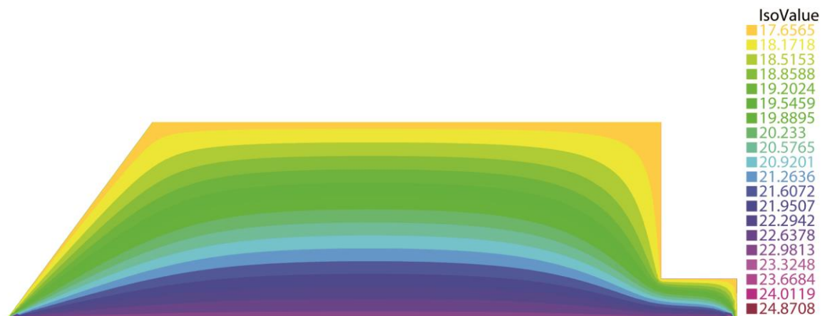
10. Results of the CFD simulation (horizontal section of the model) with air heating and solar radiation: 30 December, 8:00 h.
