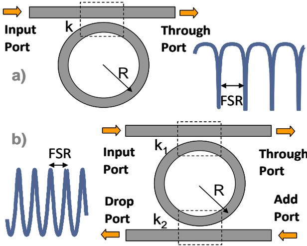
Fig. 1. Ring resonator structure: a) All-pass filter; b) Add-drop filter
