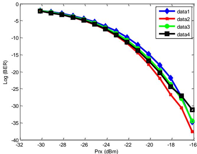
Fig. 7. BER performance of the each OFDM subchannel (data1, data2, data3, data4).
