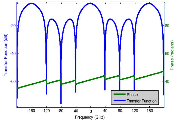
Fig. 4. Intensity transfer function and phase response of the RR-based OFDM demultiplexer for  $N=4$ .
