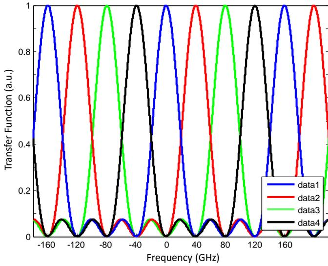
Fig. 2. Total intensity transfer function of the OFDM demultiplexer based on DIs for  $N=4$ .
