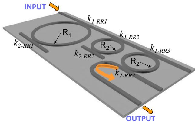
Fig. 3. Design of the OFDM demultiplexing system based on cascaded ring resonators for  $N=4$  (4 subcarriers).
