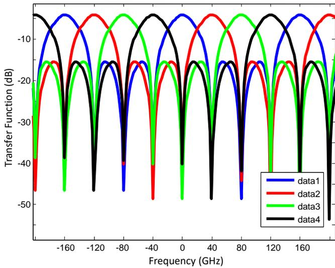
Fig. 5. Transfer function of the cascaded ring resonators for each OFDM subchannel (data1, data2, data3 and data4).
