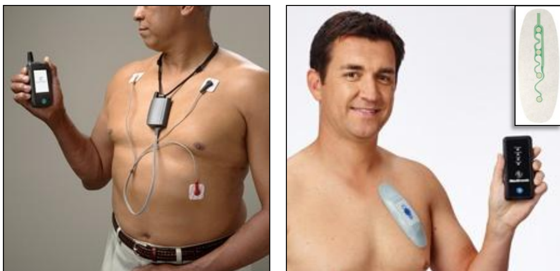
Figure 11. Mobile cardiac telemetry devices. Secondary communication devices can be noticed. Left: MCOT (CardioNet Inc.). Right: SEEQ (Medtronic), on the top right corner a detail of the electrodes embedded in the patch is shown.
