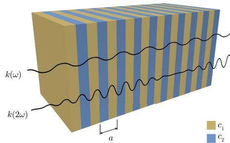
Fig. 1. Layered acoustic system with two different layers, the lattice period being  $a = a_1 + a_2$ . A second harmonic generation scheme is also represented.
