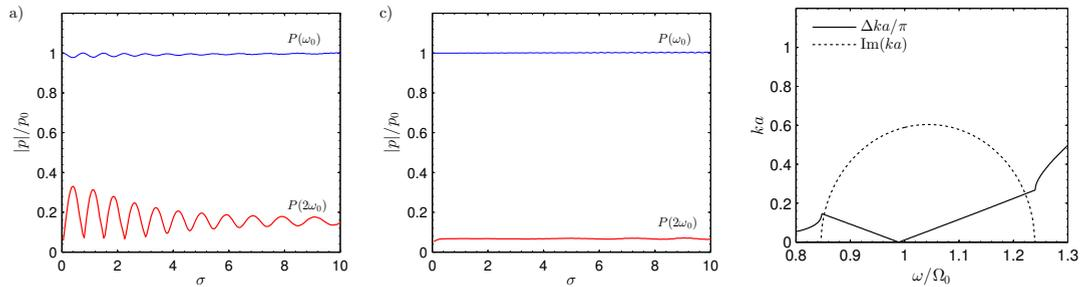
Fig. 2. For an incident wave of frequency  $\omega_0 = 0.84\Omega_0$ , evolution of the second harmonic field propagation when its frequency is (a) just above band gap, (b) in the middle of the bandgap. Results are for a layered medium with  $\alpha = 1/2$  and  $c_1/c_2 = 1/2$ . (c) Detuning of the second harmonic (continuous line) and imaginary part (dotted line) in function of the normalized frequency.
