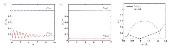
Fig. 2. For an incident wave of frequency  $\omega_0 = 0.84\Omega_0$ , evolution of the second harmonic field propagation when its frequency is (a) just above band gap, (b) in the middle of the bandgap. Results are for a layered medium with  $\alpha = 1/2$  and  $c_1/c_2 = 1/2$ . (c) Detuning of the second harmonic (continuous line) and imaginary part (dotted line) in function of the normalized frequency.
