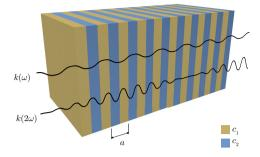
Fig. 1. Layered acoustic system with two different layers, the lattice period being  $a = a_1 + a_2$ . A second harmonic generation scheme is also represented.
