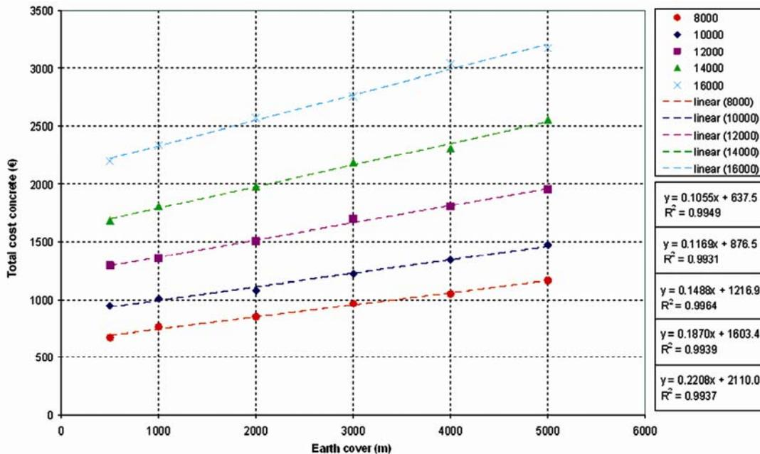
Fig. 6—Total concrete cost versus earth cover
