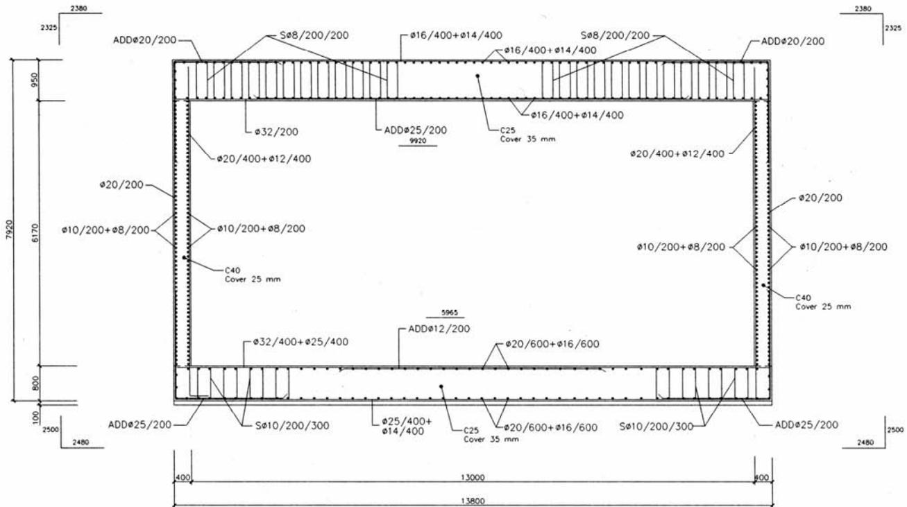
Fig. 1—Design example of RC frame bridge
