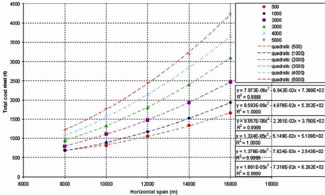
Fig. 7—Total steel cost versus horizontal span
