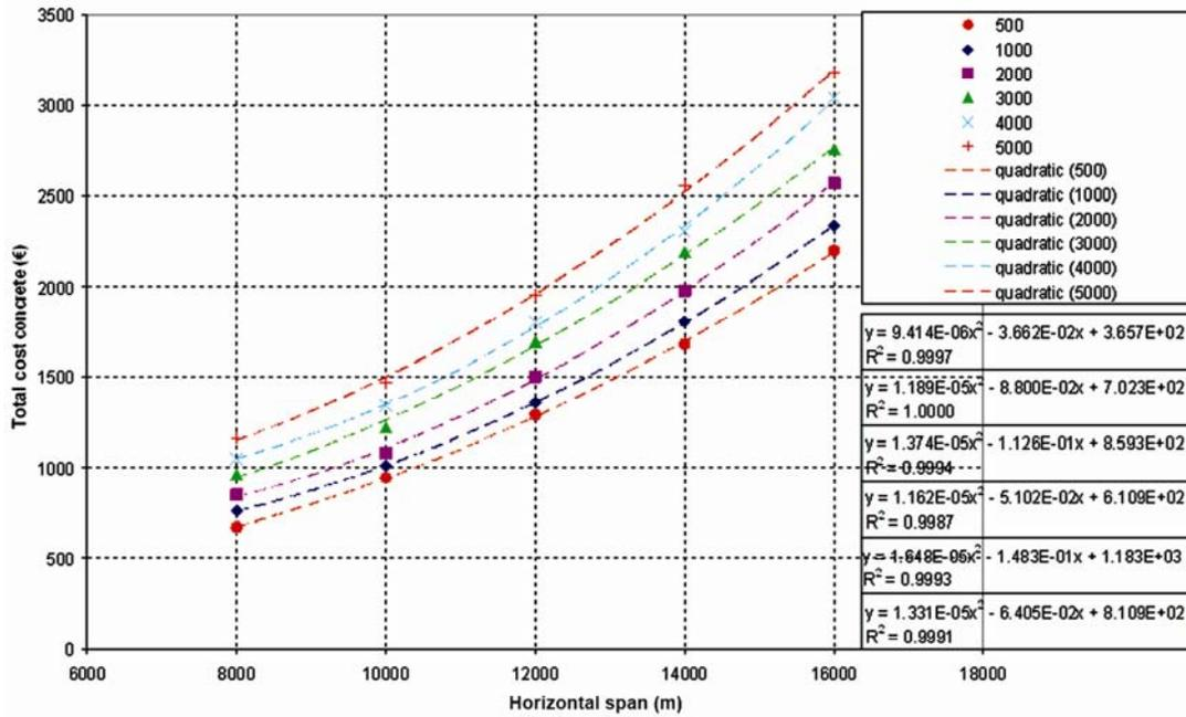
Fig. 5—Total concrete cost versus horizontal span
