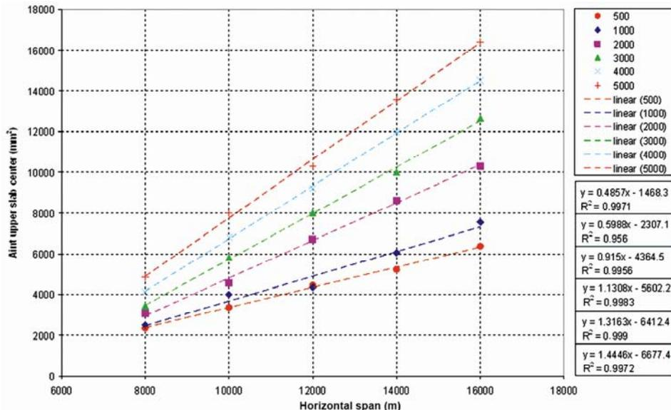
Fig. 10—Mid-span interior reinforcement area versus horizontal span
