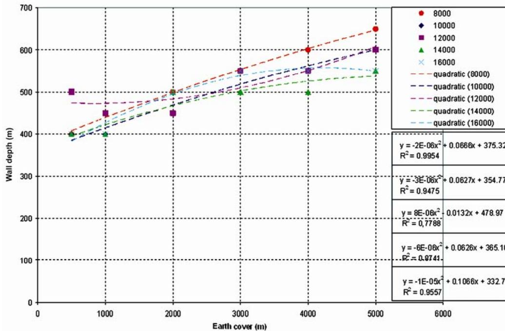
Fig. 11—Wall depth versus earth cover
