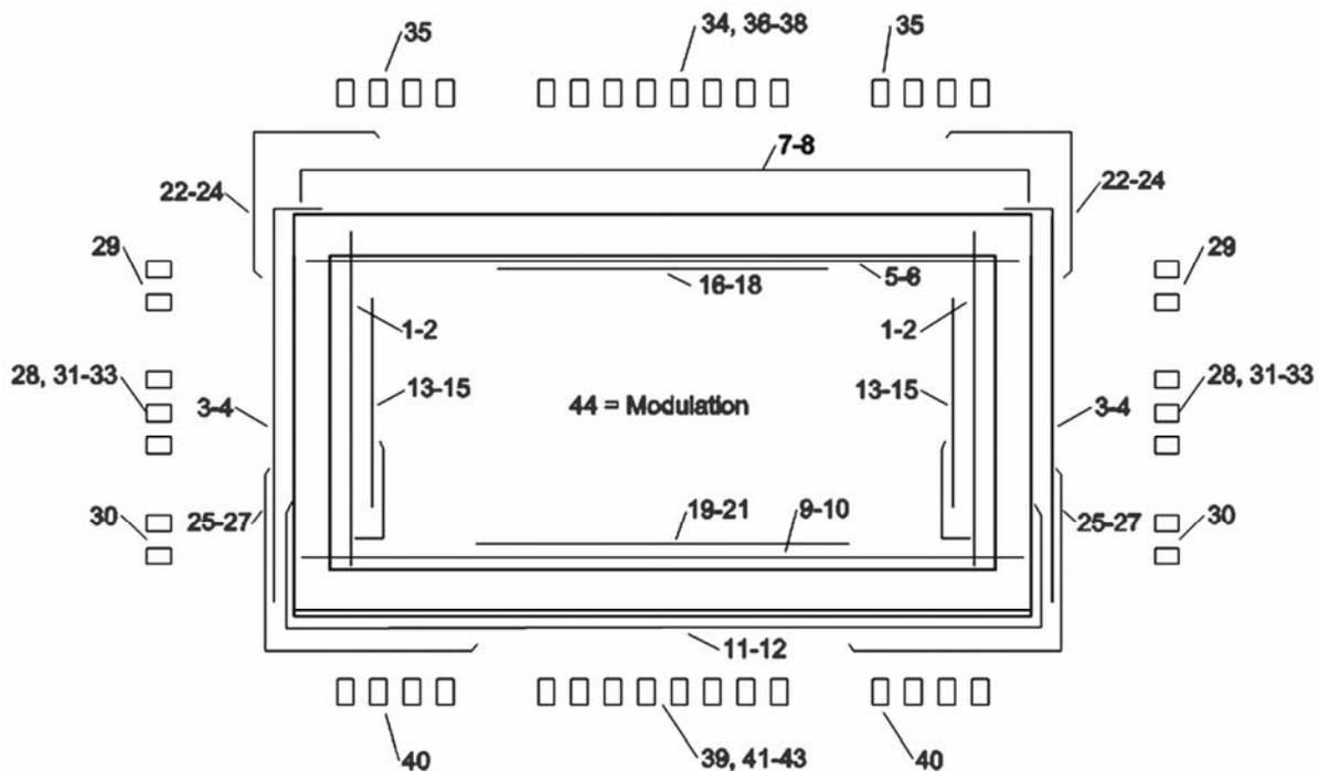
Fig. 2—Reinforcement related variables of the RC frame bridge
