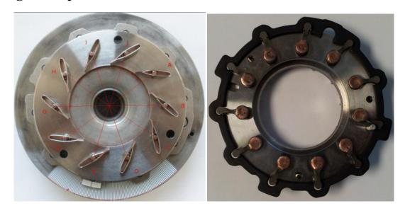
**Figure 1:** Photo of stator vanes in the fully open position. The reference radial direction is indicated for each vane.
