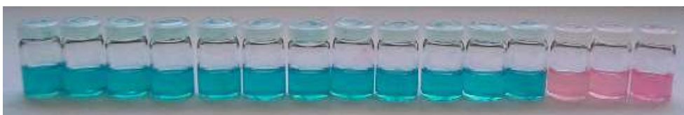
Figure 1. Photograph showing the colour change in P1-MS in the presence of amino acids and biogenic amines. From left to right: no guest, glycine, valine, leucine, phenylalanine, proline, tyrosine, arginine, tryptophan, cysteine, lysine, histidine, histamine, putrescine and cadaverine. The final solids filtered and suspended in ethylene glycol are shown.
