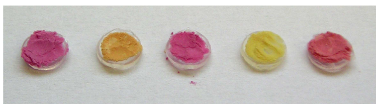
Figure 6. Colour changes observed on solid S2 upon addition of several amines. From left to right: no amine, 3,3-diphenylpropylamine, 1-methylaminopyrene, n-heptylamine and 6-amino-1-hexanol.
