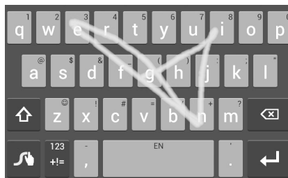
Figure 10: Swype text entry method (image from www.swype.com ).
