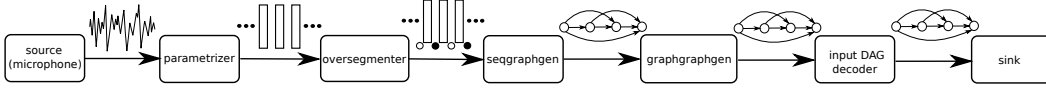
Figure 106: Dataflow architecture of a decoupled recognizer where a seq_graph_gen produces a DAG labeled with basic or sub-word units that is later converted into a DAG of lexical units to be finally combined with a LM in the DAG decoder to produces the output.
