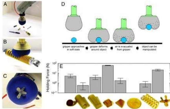
**Fig. 1** - Jamming-based grippers for picking up a wide range of objects without the need for active feedback
