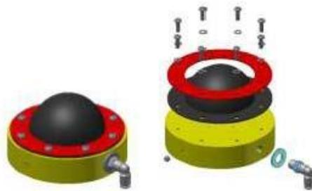
**Fig. 7** - The new concept based on the pocket with granular material: in an assembled and disassembled state
