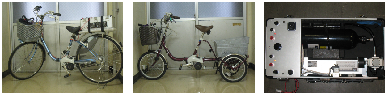
(a) Electric-assist bicycle with fuel cell generator
