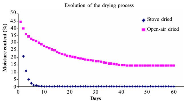
**Figure 8.** Evolution of the drying process in mandarin wood.
