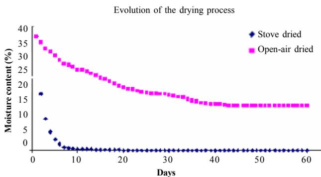
**Figure 7.** Evolution of the drying process in orange wood.
