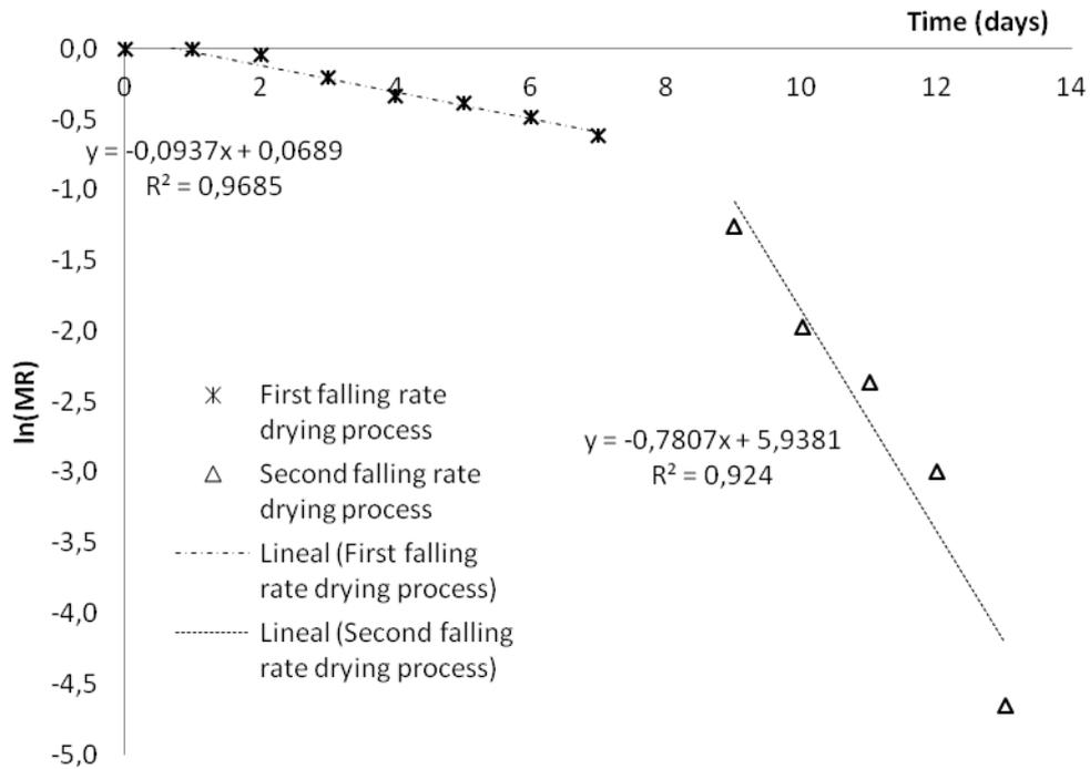
Figure 4. From Eq. (7)  $\ln(MR)$  versus time (days) for cylindrical chip corn drying of high moisture.
