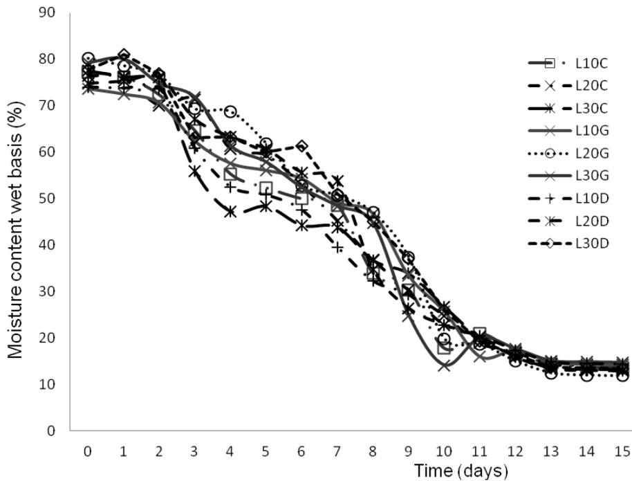
Figure 2. Comparison of drying curves for three chip sizes (L10= 10 cm length, L20= 20 cm length, L30= 30 cm length) on three drying surface (C= on cement, G= on grass, D= on dirt) in natural outdoor drying.
