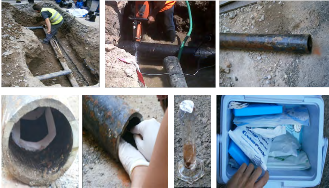
FIGURE 4.9: Biofilm sampling in Thessaloniki drinking water distribution system. Eva Ramos Martínez ©.
