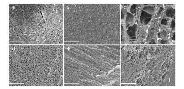
Figure 2. Cryo-SEM images of the 15% PCL/PVA scaffolds with focus on the PVA structure, after (a) 1, (b) 3 and (c) 6 cycles of freezing and thawing. The corresponding images for pure PVA gel with 1, 3 and 6 freezing and thawing cycles are shown in (d), (e) and (f) respectively. Scale bar in the pictures 10  $\mu$ m.
