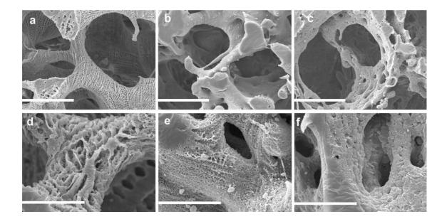
Figure 1. The PCL scaffolds showing the macro (a) 15% (b) 20% (c) 25% porosity with scale bar  $100\mu m$  and micro porosity (d) 15% (e) 20% and (f) 25% scale bar 30  $\mu m$ .
