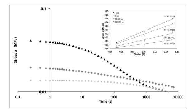
Figure 7. The logarithmic stress relaxation graphs from the compression test for the 15% PCL scaffold without (grey diamonds) and with (black triangles) PVA and the pure PVA hydrogel (light grey circles) for 15% of deformation. The inset represents the stress strain graph for 1,10,100 and 1000 s, for each time. A linear fit is represented, showing the linearity of the results.
