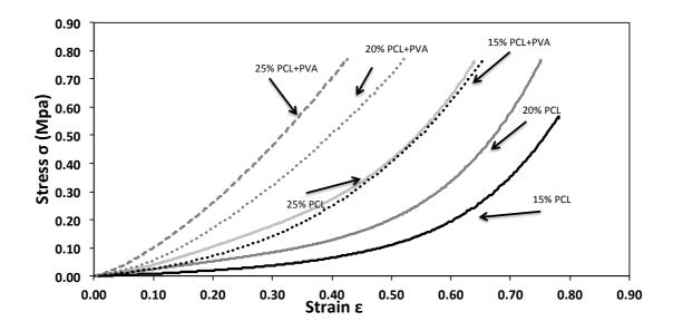
Figure 6. The loading of the PCL scaffold without (continuous line) and with PVA gel 6 cycles of f/t (dash line). The black lines is 15% PCL, the dark grey lines 20% PCL and the light grey lines 25% PCL.
