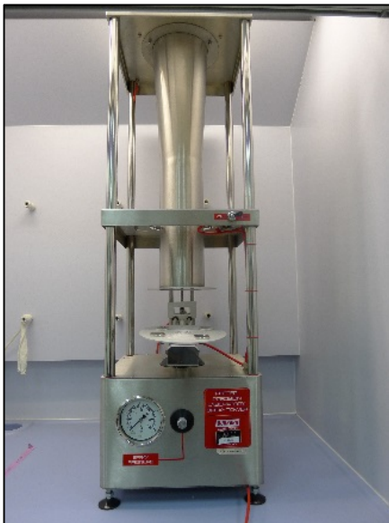
Figure 6.1. 1. Potter tower used to apply the insecticides.
