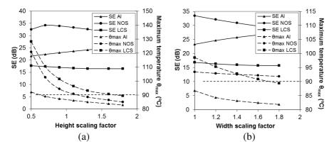
Figure 7. Evolution of the SE (at 1 m above ground surface) and the maximum temperature of the cables with (a) the height and (b) the width of the shield.
