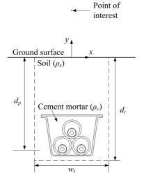
Figure 10. Underground power cables in trefoil configuration inside the shield.
