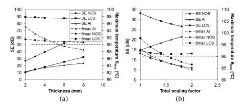
Figure 12. Evolution of the SE (at 1 m above ground surface) and the maximum temperature of the cables with (a) the thickness and (b) the size of the shield.
