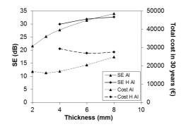
**Figure 9.** Evolution of the SE (at 1 m above ground surface) and the total cost of 100 m of shield with the thickness of the plates used in an aluminium closed shield (total scaling factor of 1.3) and a H-layout open shield (vertical plates of 1-m lenght separated by 1 m; horizontal plate of 0.9 m length and situated at 0.12 m above cables).
