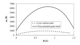
Figure 2. Relative permeability of the employed steels.
