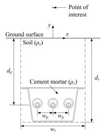
Figure 1. Underground phase conductors, screen and trench dimensions.
