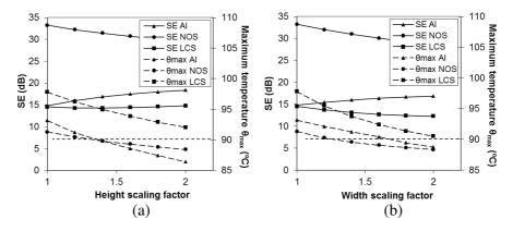
Figure 13. Evolution of the SE (at 1 m above ground surface) and the maximum temperature of the cables with (a) the height and (b) the width of the shield.
