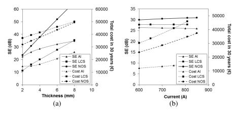
Figure 8. Evolution of the SE (at 1 m above ground surface) and the total cost of 100 m of shield (total scaling factor of 1.3) with (a) the thickness of the shield and (b) the current through the line.
