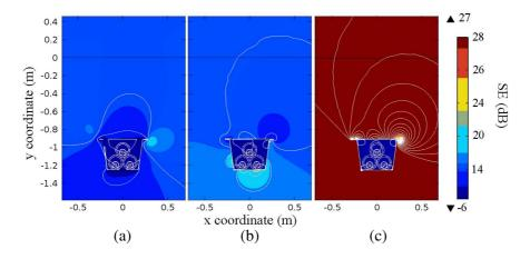
Figure 11. SE field and iso-lines for shields made of (a) aluminium, (b) low carbon steel and (c) non-oriented grain steel.
