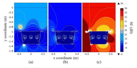
**Figure 3.** SE field and iso-lines for shields made of (a) aluminium, (b) low carbon steel and (c) non-oriented grain steel.
