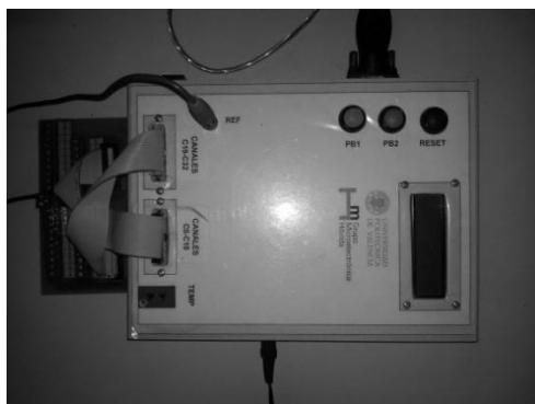
Figure 4: Data Logger on the left and the connection card on the right
