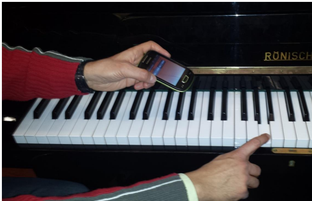
Figure 7. Photograph taken during the measurement of the frequencies of the central keys of the piano keyboard with “Frequency Analyzer” app.
