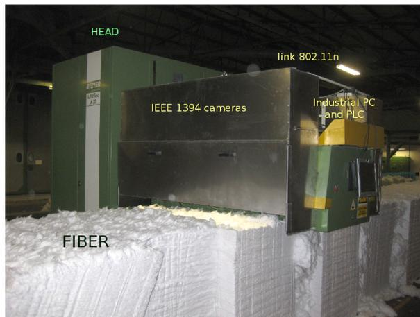
Figure 2. Head machine with the image processing system
