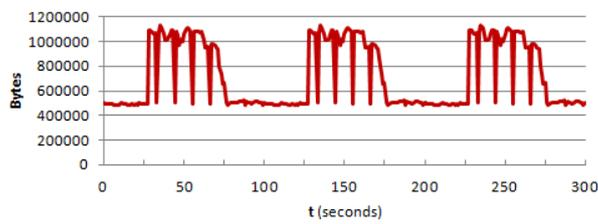
Figure 5. Image size trace used in all the experiments
