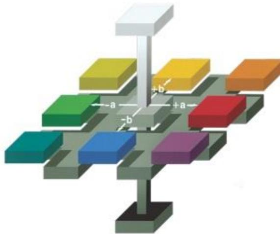
Figura 3.3. Escala de color CIE Lab. (Hunter Associates Laboratory, Inc. (2012))
