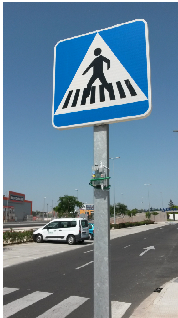
Figure 4: Traffic sign equipped with 802.11 wireless interface
