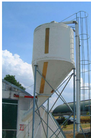
f) FRP farm silo, France
