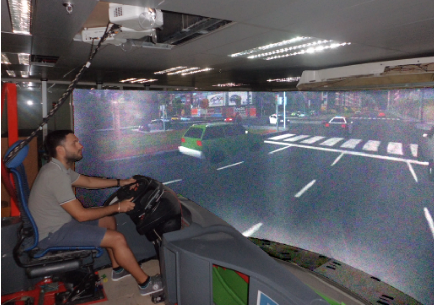
Figure 9.1: Driving simulation cabin with projection system composed by 3 projectors and a semicircular screen.
