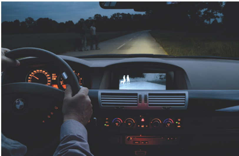
Figure 6.4: Night Vision System by BMW. Courtesy of Jan-Erik Källhammer, “Imaging: The road ahead for car night-vision”, Nature Photonics (2006).
