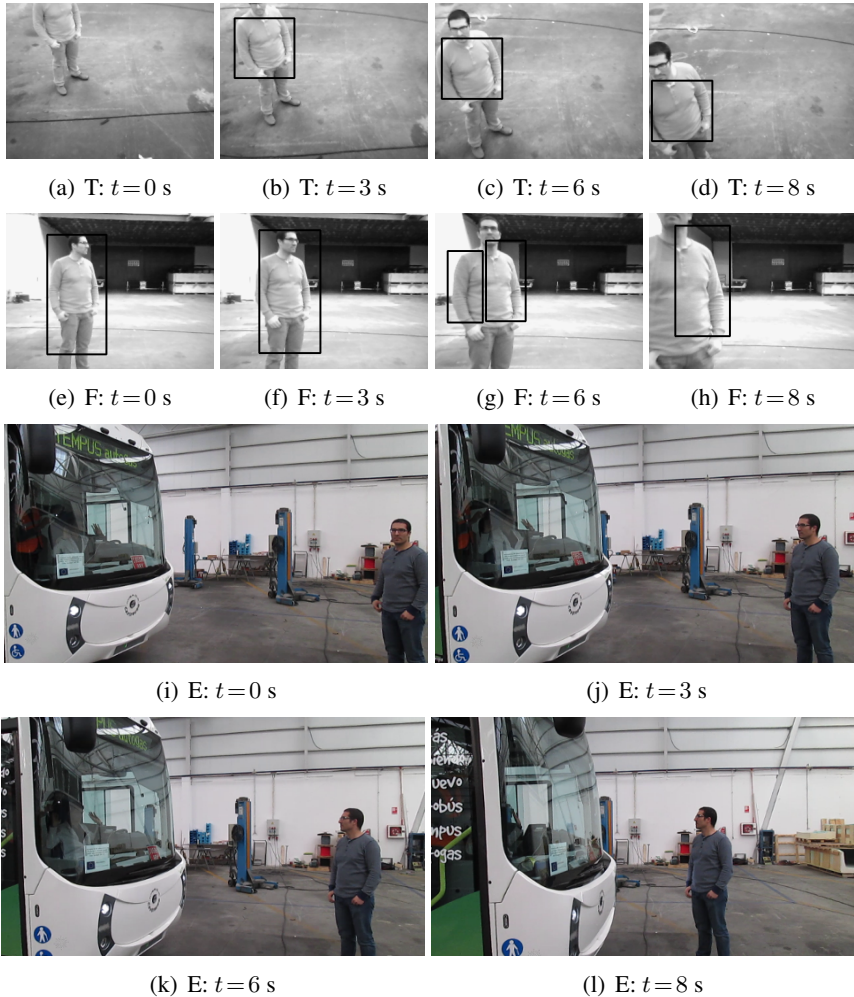
Figure 8.15: Frontal emergency experiment with images taken at different time instants from (a-c) Top center camera (T), (d-f) Front camera (F) and (g-i) Exterior view (E).
