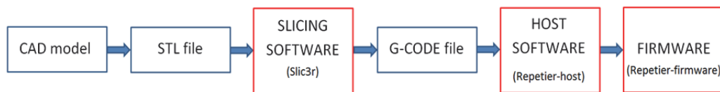
Figure 1. Workflow for printing in a 3D printer
