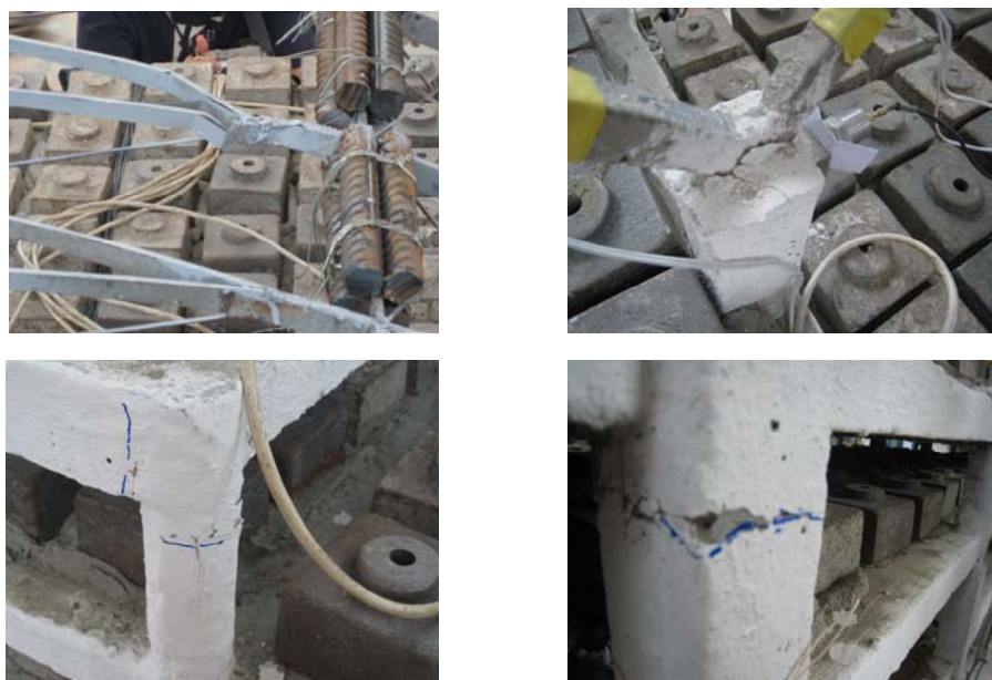
Figure 5: Cracking and failure pattern of test model
