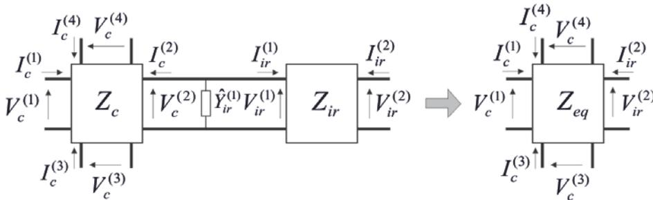
**Fig. 8.** Connection of the generalized impedance matrices related to a boxed resonator and a planar waveguide junction.
