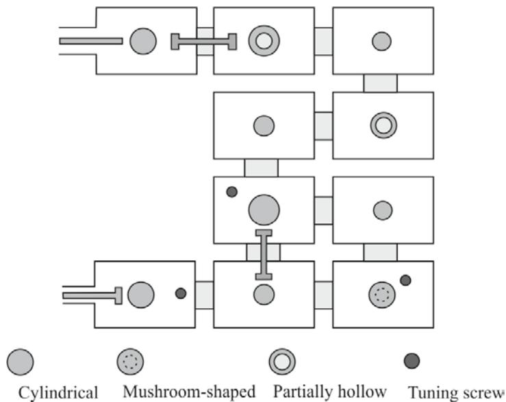
**Fig. 1.** Generic comb-line waveguide filter composed of the arbitrary connection of boxed resonators loaded with radially symmetrical metallic posts (cylindrical, mushroom-shaped and partially hollow posts). Cylindrical tuning screws are also considered in this component. The filter is excited using generalized coaxial probes, and waveguide irises with disc-ended posts (modeled as rectangular-circular coaxial waveguides) are also supported.
