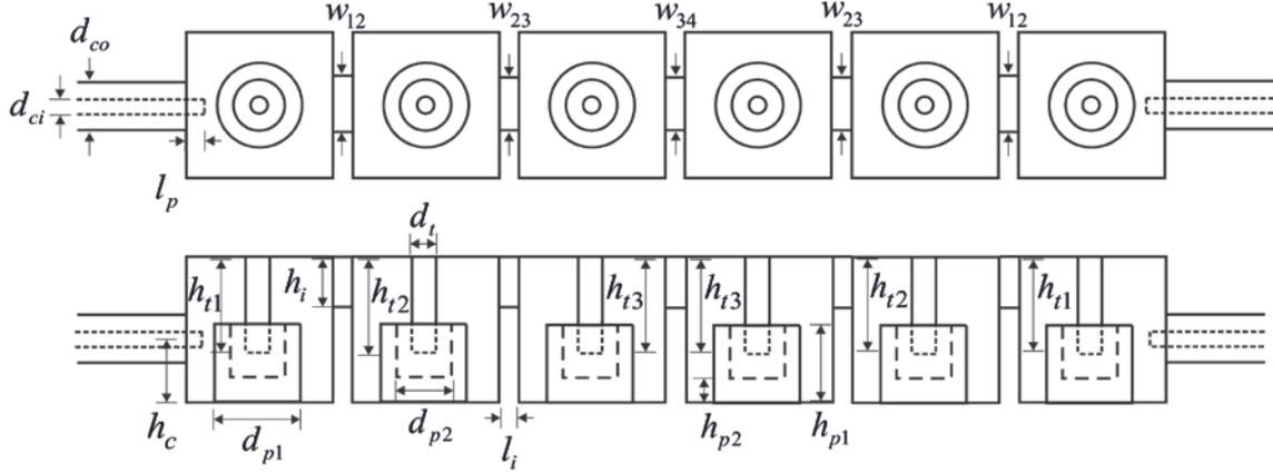
**Fig. 11.** Design of a band-pass filter composed of conductor post insert reentrant coaxial resonators. The dimensions are (all data in mm):  $d_{co} = 4.2$ ,  $d_{ci} = 1.27$ ,  $l_p = 3.817$ ,  $w_{12} = 9.208$ ,  $w_{23} = 8.019$ ,  $w_{34} = 7.862$ ,  $d_{p1} = 12.0$ ,  $d_{p2} = 10.0$ ,  $h_{p1} = 10.5$ ,  $h_{p2} = 3.0$ ,  $h_{t1} = 12.344$ ,  $h_{t2} = 12.509$ ,  $h_{t3} = 12.533$ ,  $d_t = 3.0$ ,  $h_c = 9.5$ ,  $l_i = 2.0$ ,  $h_i = 8.0$ .
