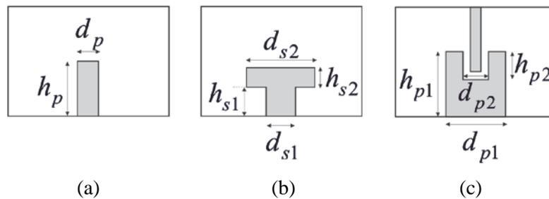
**Fig. 2.** Radially symmetrical partial-height metallic posts supported by the implemented CAD tool: (a) cylindrical, (b) mushroom-shaped, and (c) partially hollow post. Note that a cylindrical tuning screw has been included in (c) to cope with the analysis of conductor post insert reentrant coaxial resonators, and that an arbitrary number of radially symmetrical tuning screws can be added in the cavities of (a) and (b).
