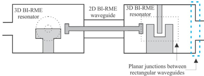
**Fig. 5.** 2D view of the planar waveguide junctions present in Fig. 4.
