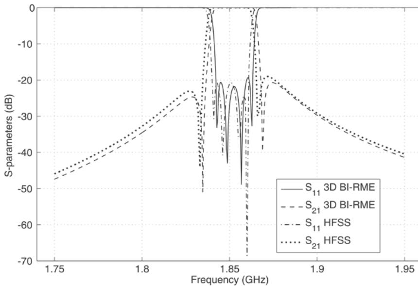
**Fig. 14.** Scattering parameters of the L-band filter designed in Fig. 13.
