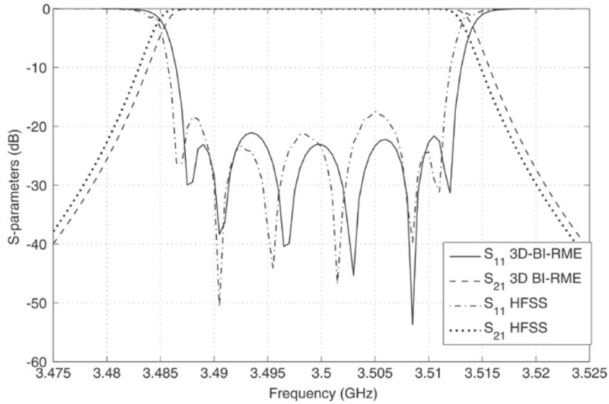
**Fig. 12.** Scattering parameters of the S-band filter designed in Fig. 11.
