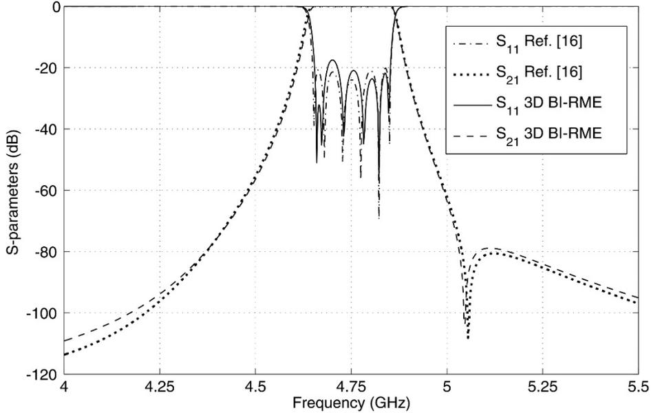
**Fig. 10.** Scattering parameters of the folded comb-line filter with cross-coupling designed in reference [16].
