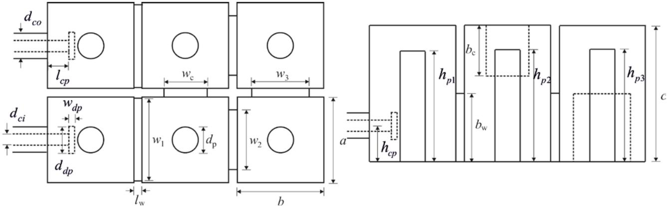
**Fig. 9.** Design of a folded comb-line filter with a cross-coupling configuration [16]. The dimensions are (all data in mm):  $d_{co} = 3.0$ ,  $d_{ci} = 1.3$ ,  $l_{cp} = 2.5$ ,  $w_{dp} = 0.6$ ,  $d_{dp} = 3.2$ ,  $h_{cp} = 4.21$ ,  $h_{p1} = 13.015$ ,  $h_{p2} = 13.163$ ,  $h_{p3} = 13.22$ ,  $d_p = 3.0$ ,  $w_1 = 9.7$ ,  $w_2 = 6.99$ ,  $w_3 = 6.68$ ,  $w_c = 5.0$ ,  $b_c = 6.0$ ,  $b_w = 8.0$ ,  $l_w = 1.0$ ,  $a = b = 10.0$ ,  $c = 16.0$ .
