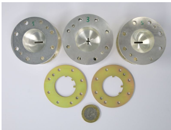
Figure 4: Detailed view of the pieces composing the CWDM filter in Fig. 3.
