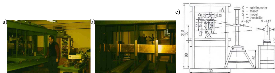
Figure 5: View on stand for bending-torsion loading of rectangular brazen cantilevers a); four steel frames for measurements of displacements; at left fastening and hinge (breaking point) b); a) Scheme of optical observation for circuital and longitudinal displacements c)
