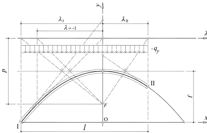
Figure 4: Parabolic arch with constant cross-section vertically loaded.
