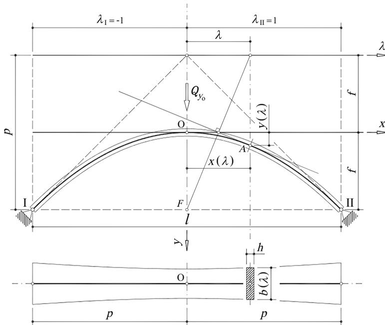
Figure 2: Hinged parabolic arch with hyperbolic variable cross-section.
