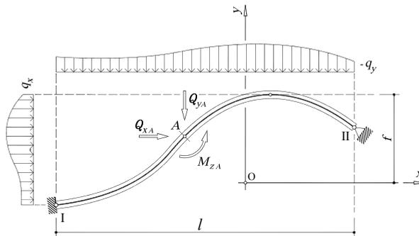
Figure 1: Generic arch with punctual and distributed load.
