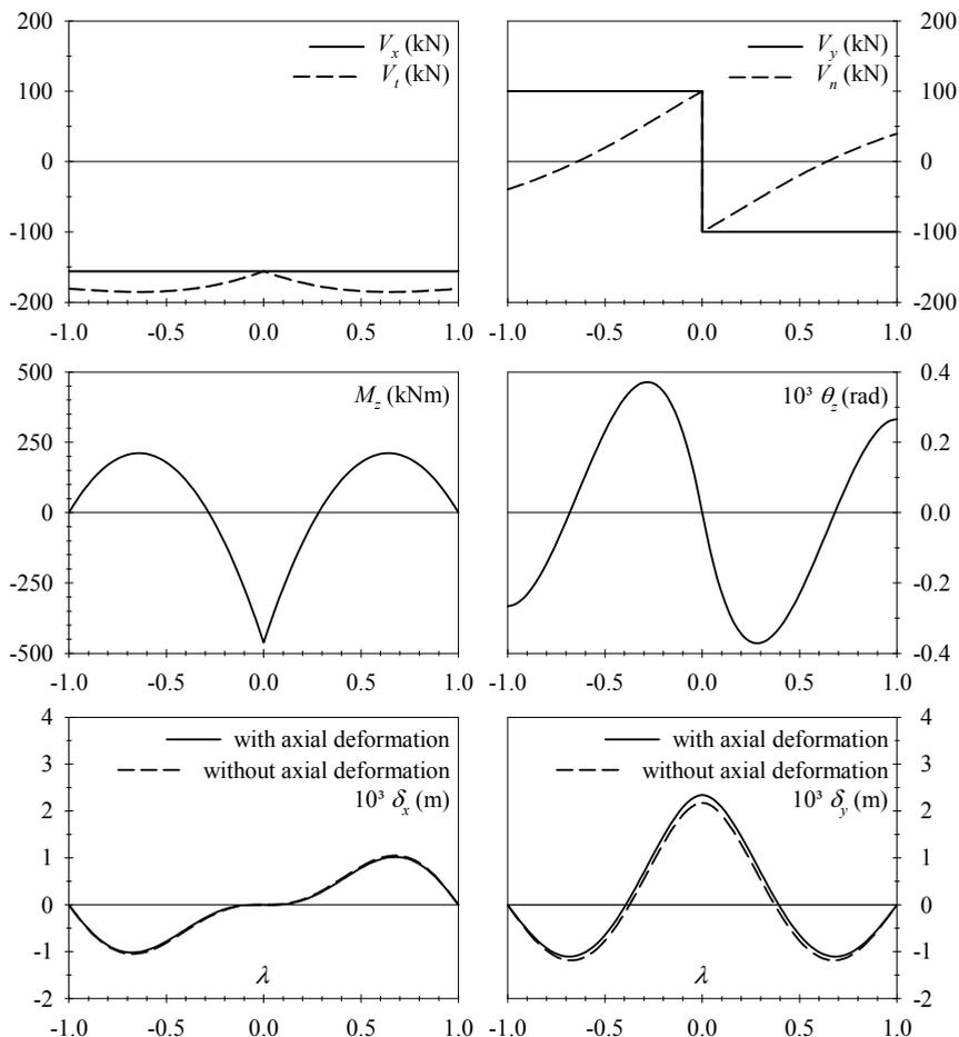
Figure 3: Forces, moment, rotation and displacements of the parabolic arch.
