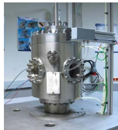
Figure 1. High Pressure-High Temperature test rig
