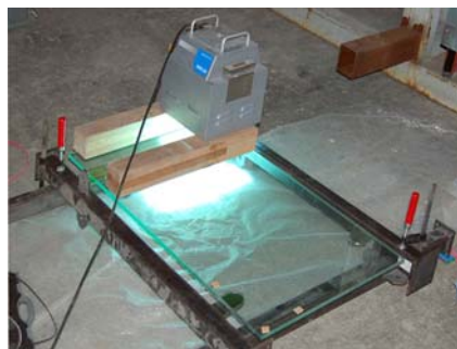
Figure 3+4: Safety barrier. The curing process with a special lamp and the simulation of static loads by sand sacks
