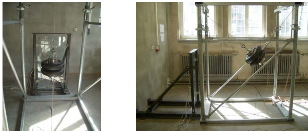
Figure 5+6: Pendulum impact test of the safety barrier
