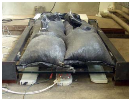
Figure 3+4: Safety barrier. The curing process with a special lamp and the simulation of static loads by sand sacks
