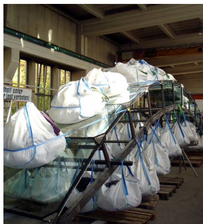
Figure 17 and 18: Digital displacement transducer in the middle of the girder and loaded girder
