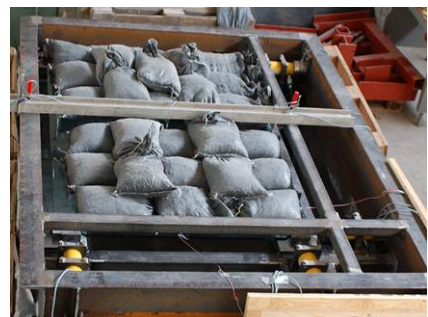
Figure 9+10: Arrangement of testing devices and pre-load by sand bags
