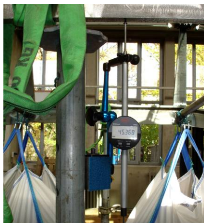
Figure 17 and 18: Digital displacement transducer in the middle of the girder and loaded girder
