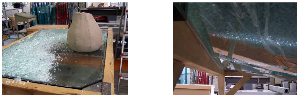
Figure 14+15: Cleaned dropping location and support by the tension rods
