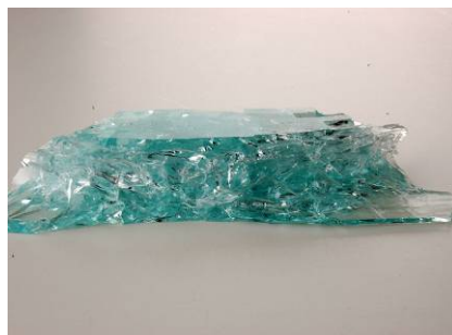
Figure 12+13: Begin of breakage and Fracture pattern
